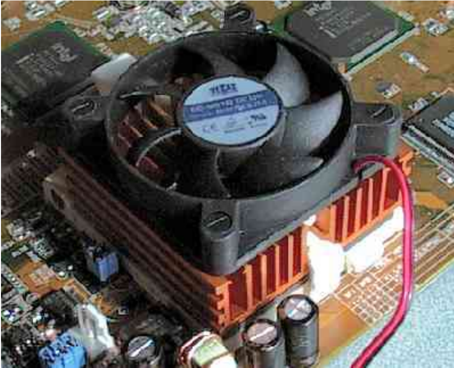
Pentium with fan. Photo taken with Canon Powershot 600. JPG-file 1:30, 32 KB.
